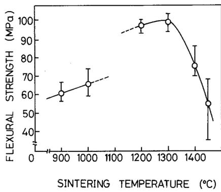
Figure 1 Flexural strengths of cordierite ceramics.
