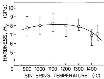
Figure 4 Vickers hardness of cordierite ceramics.
