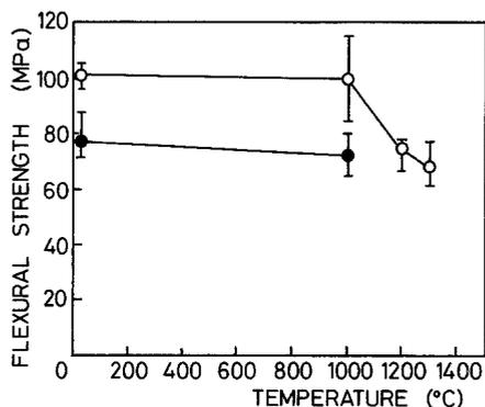
Figure 8 High-temperature flexural strengths of  $\alpha$ -cordierite ceramics.
