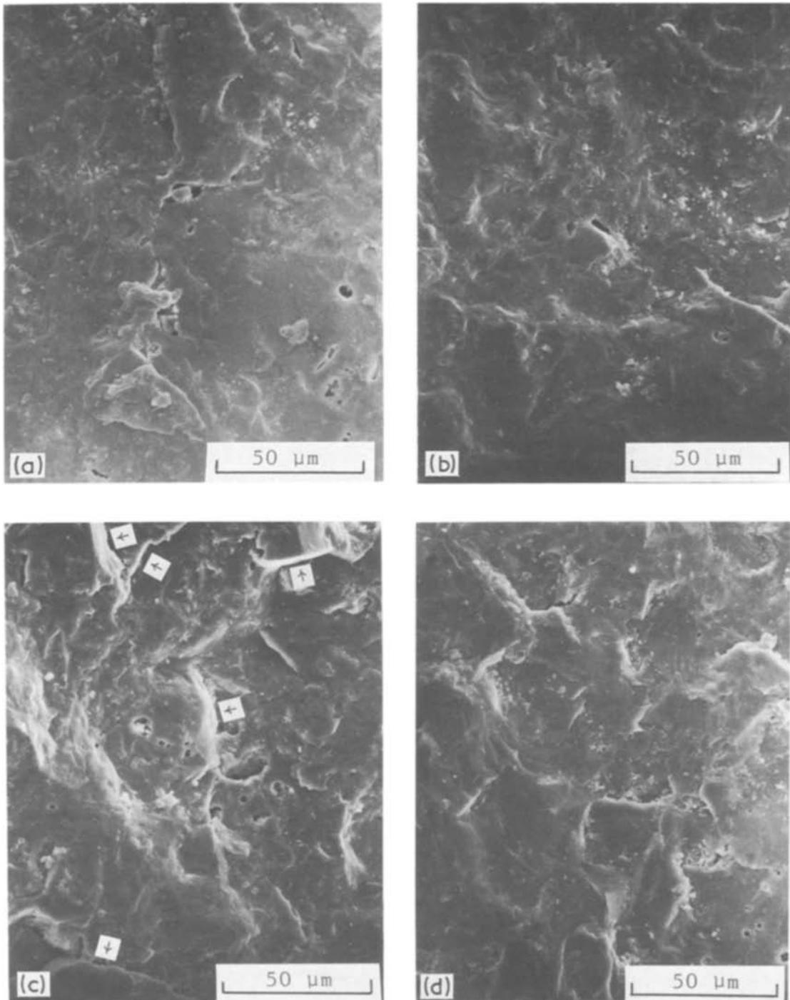
Figure 2 SEM images of the fractured surfaces of cordierite ceramics sintered at (a) 900°C, (b) 1000°C, (c) 1100°C, (d) 1200°C, (e) 1300°C, (f) 1400°C, (g) 1450°C.
