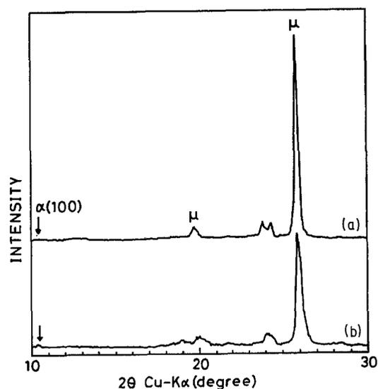
Figure 3 X-ray diffraction patterns of the cordierite powders. (a) Calcined at 980°C for 2 h, (b) calcined at 980°C for 160 h.
