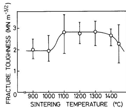
Figure 6 Fracture toughness of cordierite ceramics.
