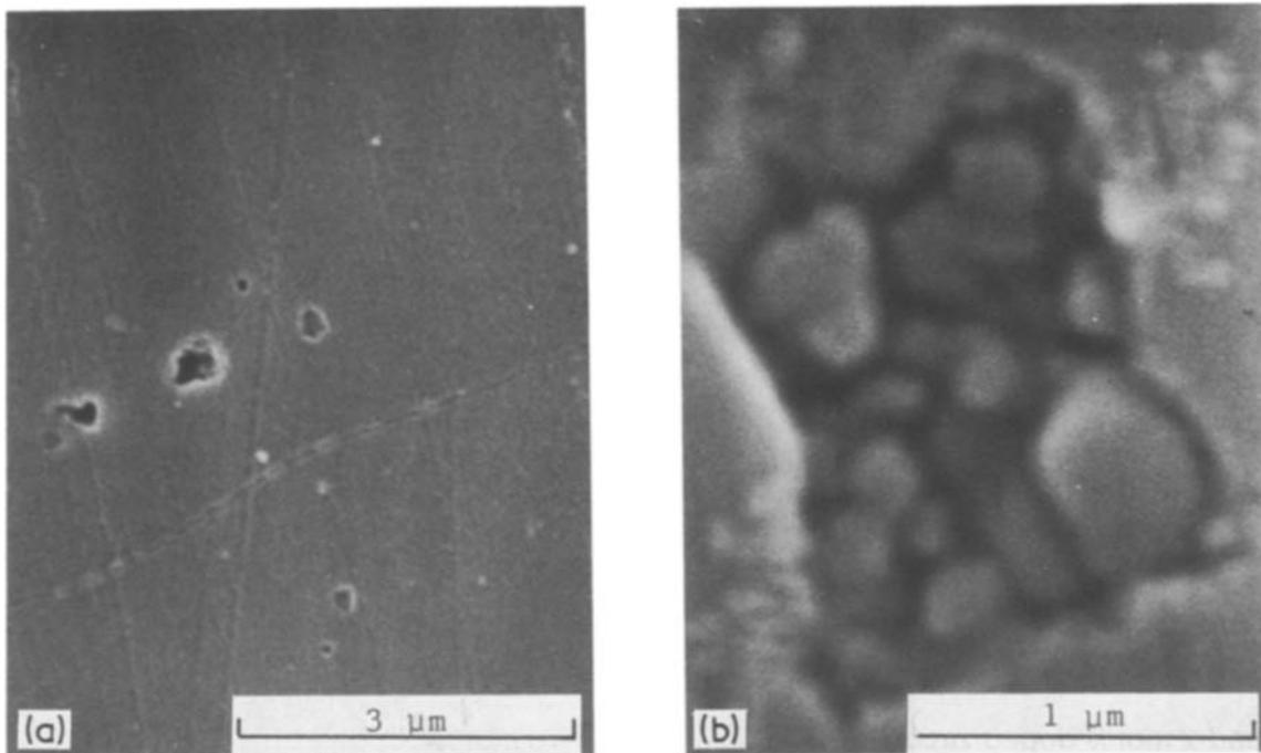
Figure 7 High-magnification SEM images of the polished and chemically etched surface of  $\alpha$ -cordierite ceramics sintered at 1300°C for 2 h.
